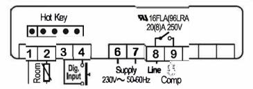
NOTE: The compressor relay is 20(8)A or 8(3)A depending on the model. NOTE: 120Vac connect to 6.7.
